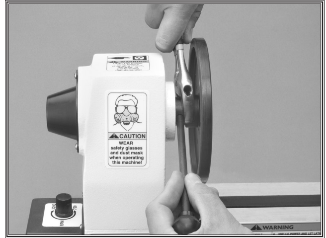
Figure 11. Tightening face plate to headstock spindle.
